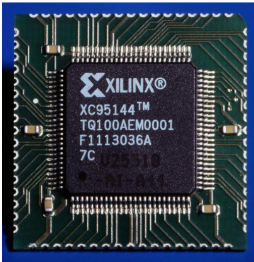
PCB carrier with CPLD as ASIC replacement
