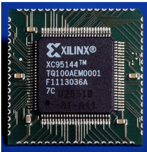
PCB carrier with CPLD as ASIC replacement
